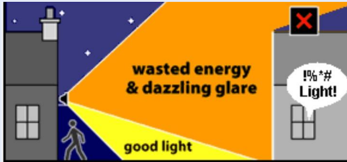
BADLY AIMED 500W HALOGEN FLOODLIGHT
