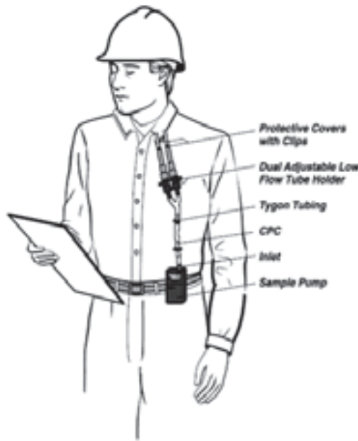
Worker wearing sampling pump and two tubes side-by-side for simultaneous tube sampling
